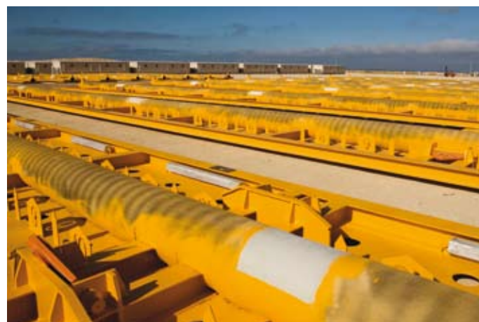
Displacement initiator frames for subsea pipelines were also fabricated at PIC's facility and transported to the CUF for Woodside's Pluto Project.
