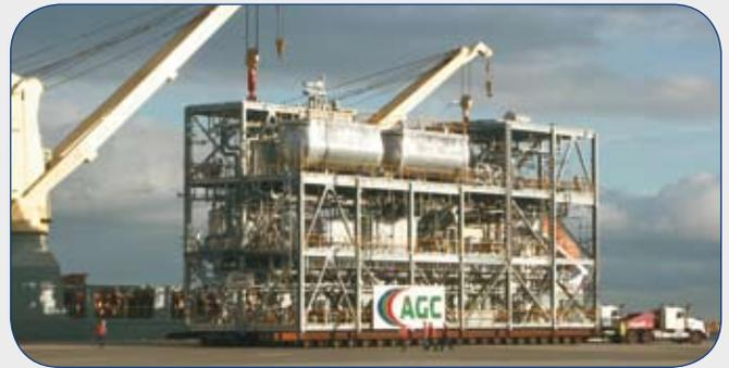
The 420 tonne biodiesel plant being loaded for marine transport to Darwin.
